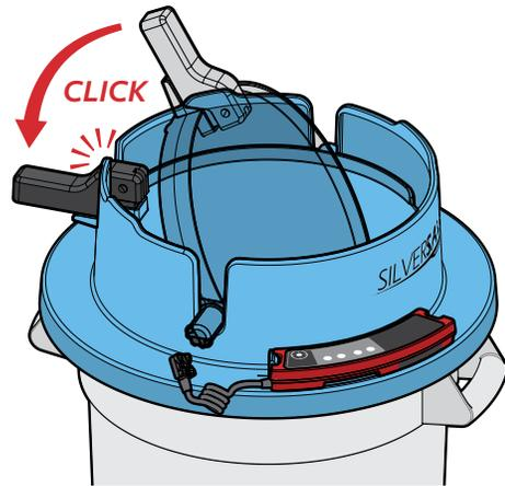
5. Connect the Tray to the Control Box by snapping the Magnetic Connector onto the Connector Pads on the Tray Axle.
